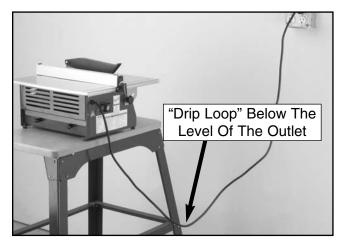
Figure 4. Correct cord positioning.
